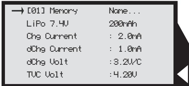
The Memory Name menu is where the parameters for charging or discharging batteries are defined. The corresponding settings are then stored in the memory. (See Page 14 for setting process parameters)
