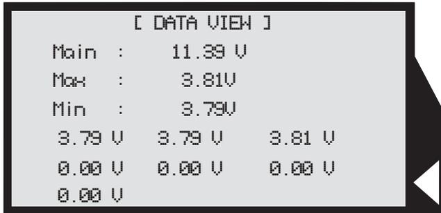
The Data View menu displays information pertaining to the charging and discharging processes of a Lithium chemistry battery. When a balancing cable is attached, the screen will also display the voltage of the individual cells as well as the highest and lowest cell value.
