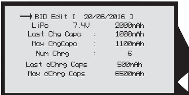
The BID Information screen displays a variety of data such as last charge capacity, maximum charge capacity, the number of discharge cycles, last discharge capacity and maximum charge capacity.
