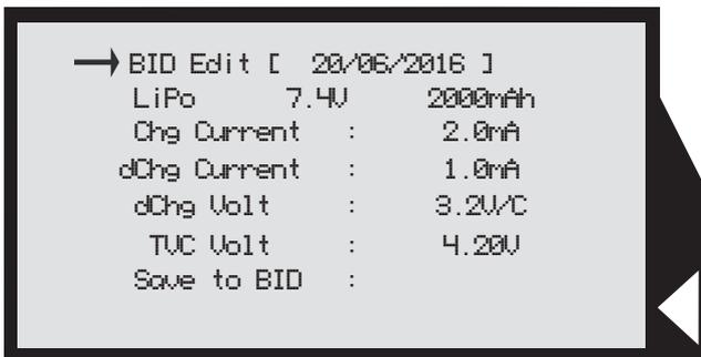
The BID chip or Key is programmed just like a memory slot. Refer to page 14 to set the charge or discharge parameters. Once set, use the + and – buttons to scroll to Save to BID and press START/ENT to write the settings to the BID Chip or Key already connected.
