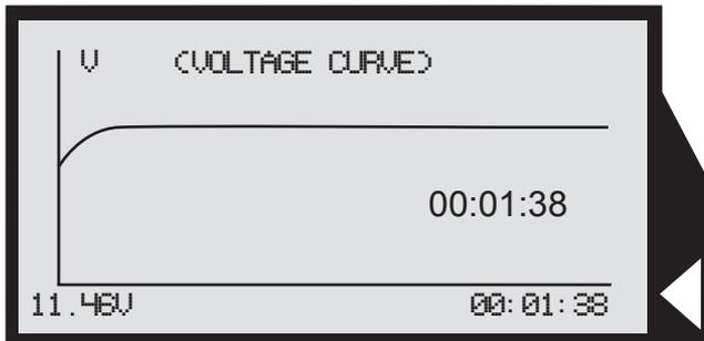
The voltage curve screen shows the voltage curve during the charge or discharge process. Also shown is the actual voltage as well as elapsed time.
